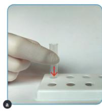
Remove the cover and Insert the extraction tube into the bottom of the bracket
