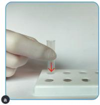
Insert the extraction tube into the bottom of the bracket
