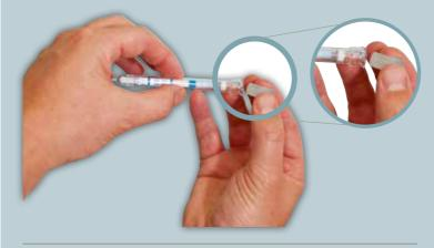
3. Drop it into the bottom of the test stand G using your finger.
