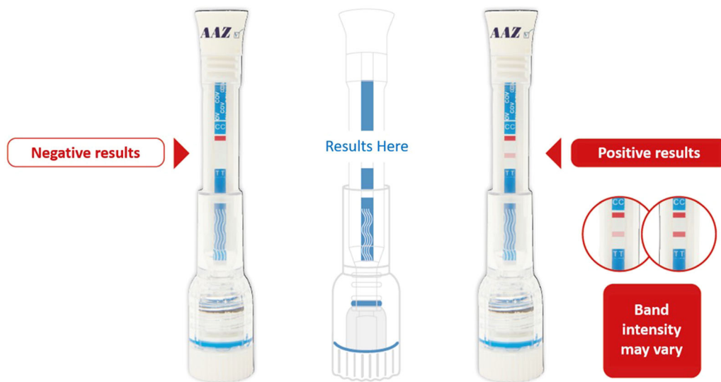
FIGURE 1 Visual appearance of the COVID-VIRO ALL IN ® test device and representation of the potential results.
